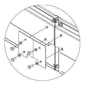
6. Attach entire assembly to factory brackets using (4) M6 x 20 pan head screws and (4)<sup>1</sup>/<sub>4</sub>" flat washers. See below, arrows indicate direction of factory brackets.
