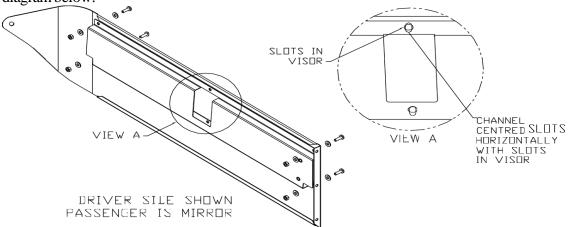
5. Fasten center bracket to channels using (4) <sup>1</sup>/<sub>4</sub>-20 hex bolts and (4) <sup>1</sup>/<sub>4</sub>" lock washers. Leave slightly loose to allow for adjustment. Seebelow. Page 1 of 2
