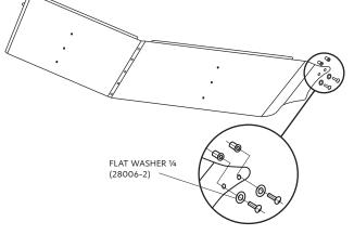
\* Depending on the year of the truck, holes may need to be drilled on the front of the cab for proper installation
